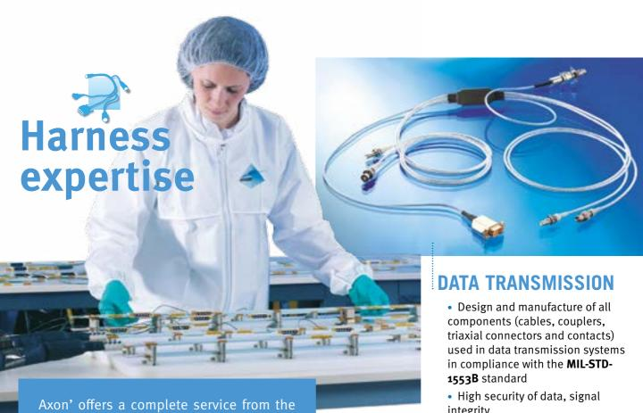
choice of material or components, to the design, routing, manufacturing, test and qualification of your products. 2D or 3D cabling boards can be developed to ensure perfect integration at the customer's facilities, for example where tolerances on length or the required routing are very tight.
